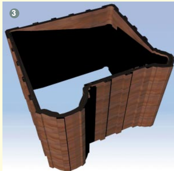
(3) The result of lofting the traced image, with a stone material mapped on to its surface
